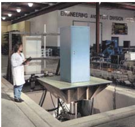
Seismic tables such as this at the Jefferson Technology Center simulate earthquakes so that materials can be tested for strength and endurance under such difficult-to-replicate conditions.
